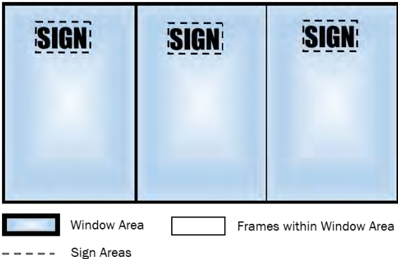
Figure 506-13 Window with more than one frame
