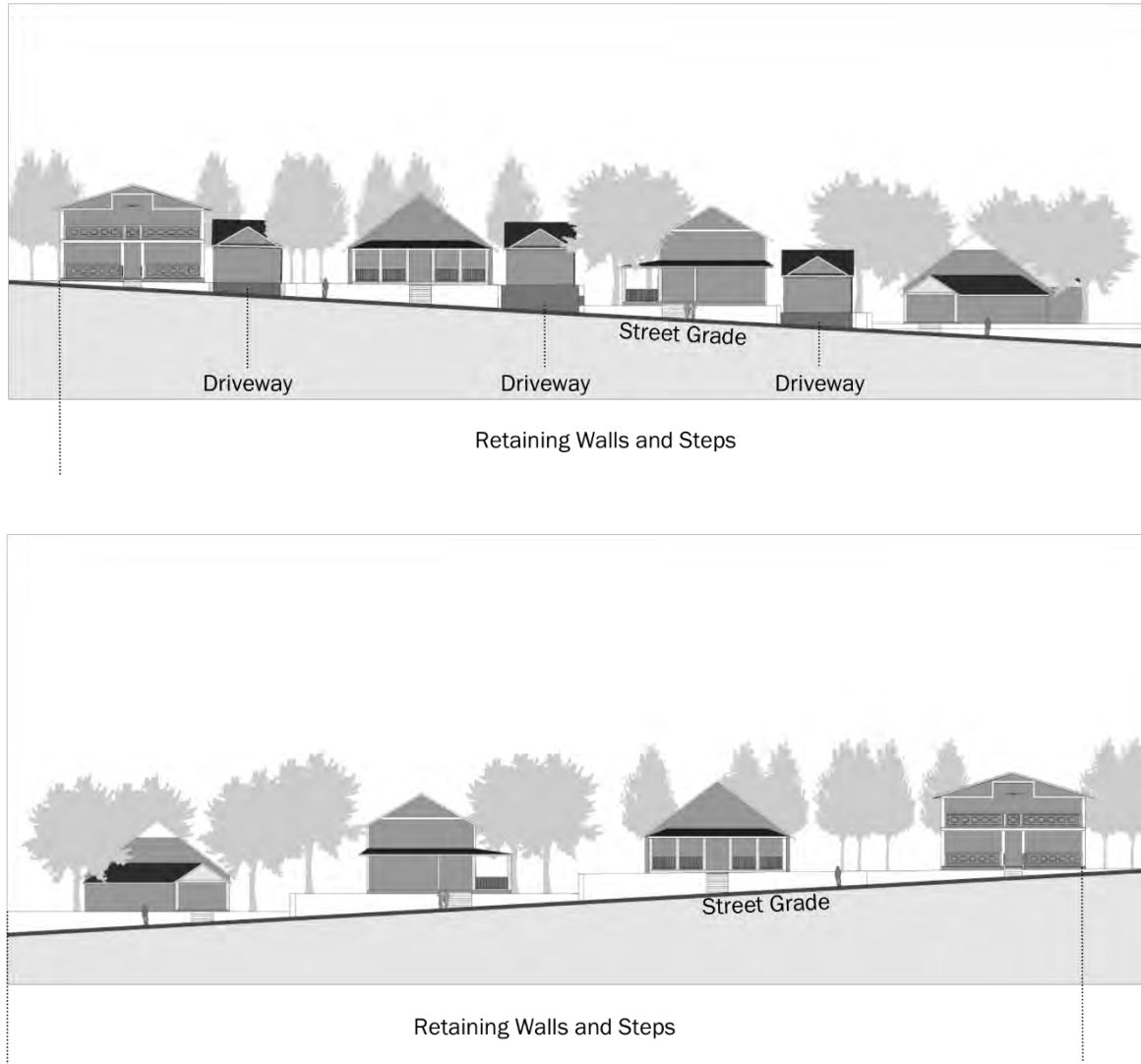
Figure 227-5 Cross-Slope Lots: Front-Loaded and Alley-Loaded
